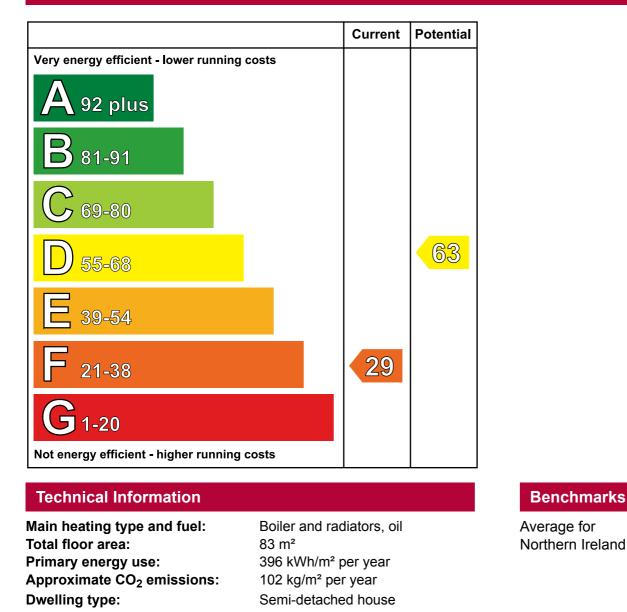
The primary energy use and  $CO_2$  emissions are per square metre of floor area based on fuel use for the heating, ventilation, hot water and lighting systems. The rating can be compared to the benchmark of the average energy efficiency rating for the housing stock in Northern Ireland.
